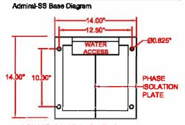
A PHASE ISOLATION PLATE SHALL BE INCLUDED FOR ALL PEDESTALS CONTAINING TWO WIRE FEEDS OF DIFFERING VOLTAGES. NO ISOLATION PLATE IS INCLUDED FOR SINGLE FEED PEDESTALS.
